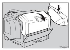
If the misfed paper is in the front of the photoconductor unit, carefully pull it out.
